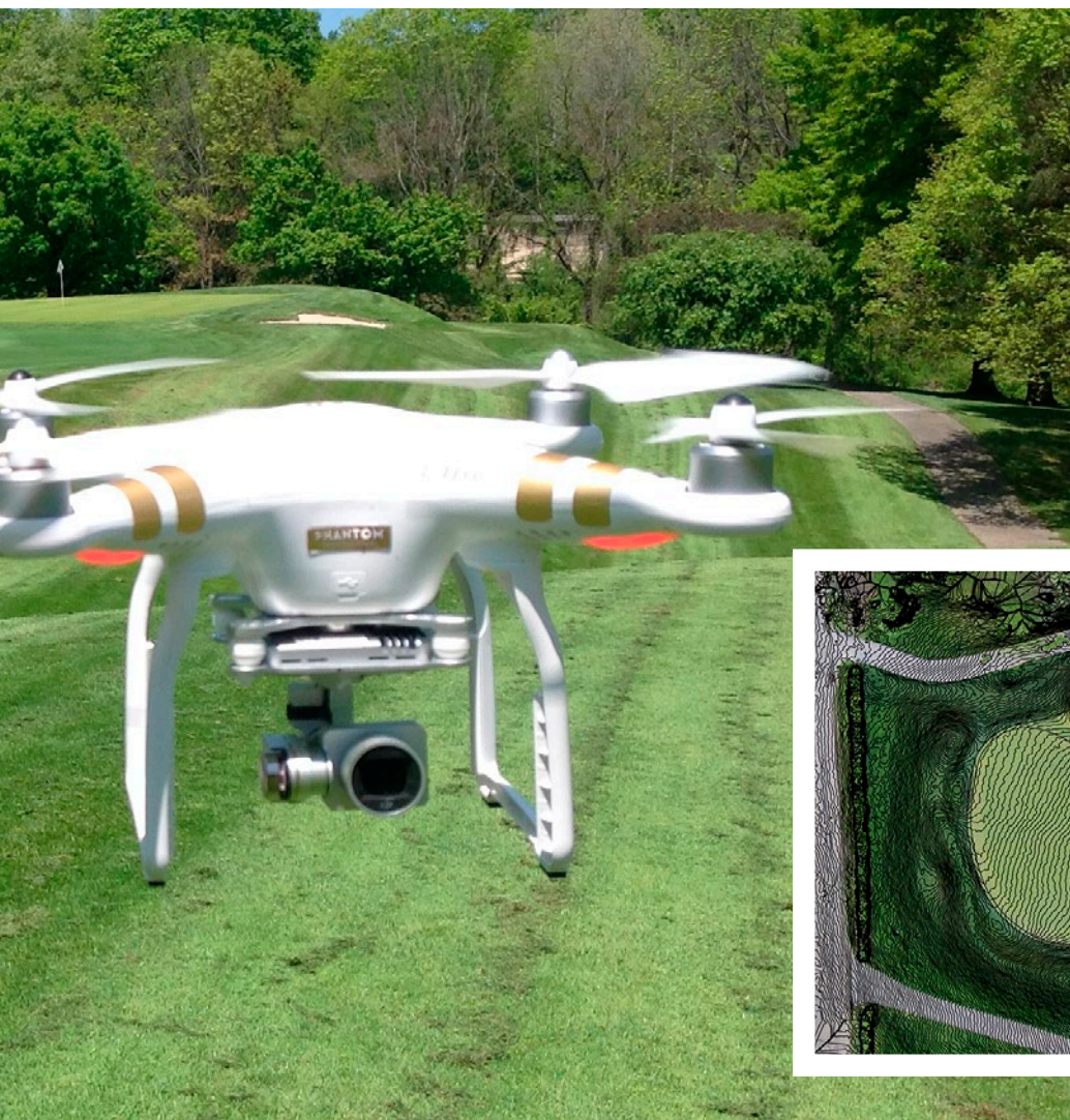
Jim Cervone, ASGCA, considers the drone 'a wonderful addition to the toolbox' and has used it to produce topographic maps with one-inch contour precision (inset)
