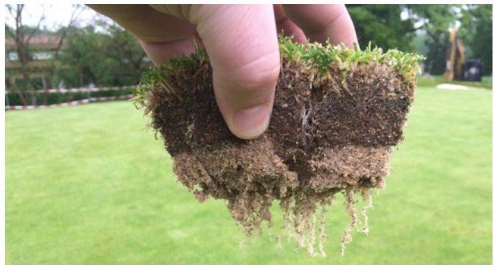
A rootzone plug from the 14th green shows the integration of the existing grass with the new sand/Profile mix – a few weeks after the existing green sod was laid over the new rootzone
