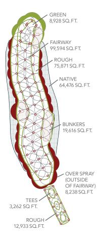
The next issue is a loss of irrigation uniformity due to the difference in the interior sprinkler pattern vs. the exterior sprinkler pattern. You can see that the interior pattern, where you have three or four sprinklers contributing to the coverage, provides excellent uniformity, and thus a very high Scheduling Coefficient (Sc) of 1.2 is achieved.
